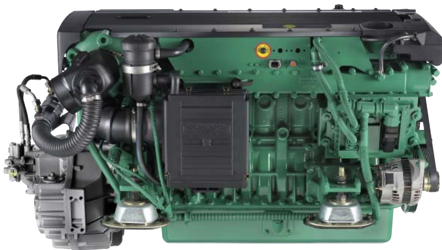
D6-370 with HS80AE reverse gear
